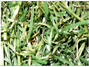
Fibers Taken from Control Area of Specimen – Not Exposed to Mechanical Abrasion
